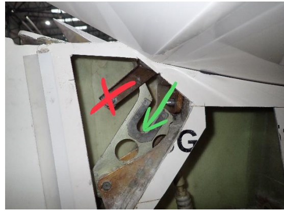
Image 2 Disconnected elevator control
