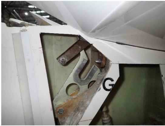
Image 1 Disconnected elevator control
